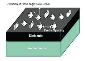
Figure 1: Schematic diagram of conventional Si BioFET structure.
