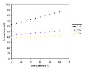
Figure 4: p-Si nanowire simulation of conductance vs. binding efficiency with 1 micron gate length and 1 nm oxide layer thickness at a drain voltage of 1V.
