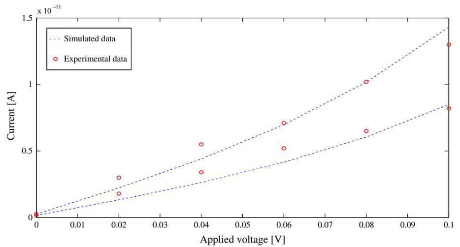
**Fig. 9** Comparison of simulated and measured [7]  $Na^+$  current through a KcsA channel for a 500 mM bath concentration
