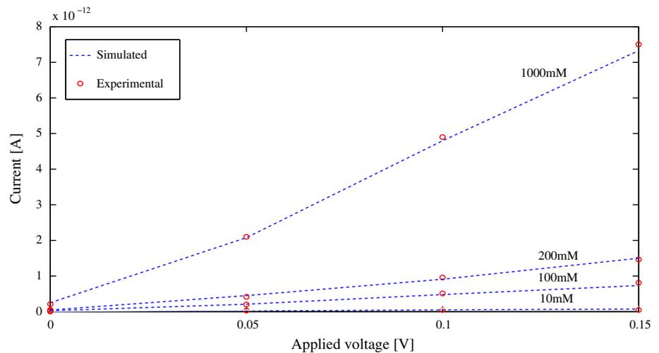
**Fig. 5** The measured [14] and simulated  $\text{Na}^+$  currents through the Gramicidin A channel for positive and negative applied voltages
