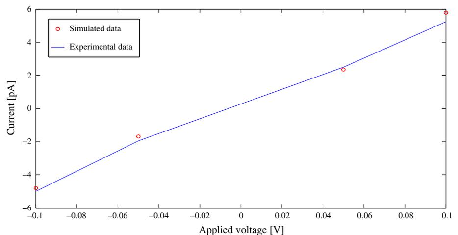
**Fig. 6** The simulated versus the experimental [2]  $K^+$  current for different applied voltages
