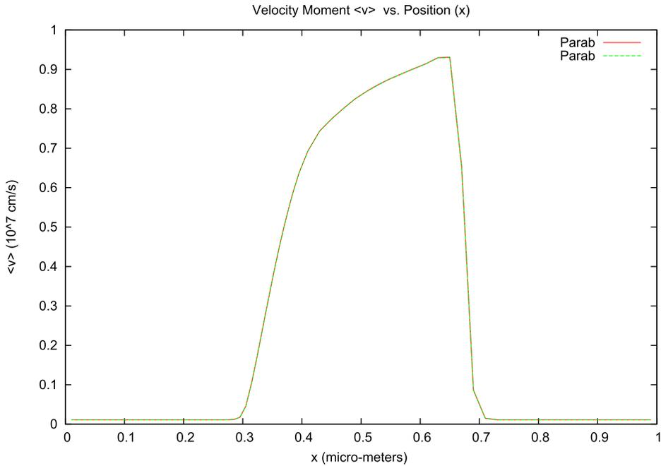
Fig. 12. Velocity  $v(x, t_0)$  for a 1  $\mu\text{m}$  diode, 0.5 V bias, and  $t_0 = 10.0$  ps.
