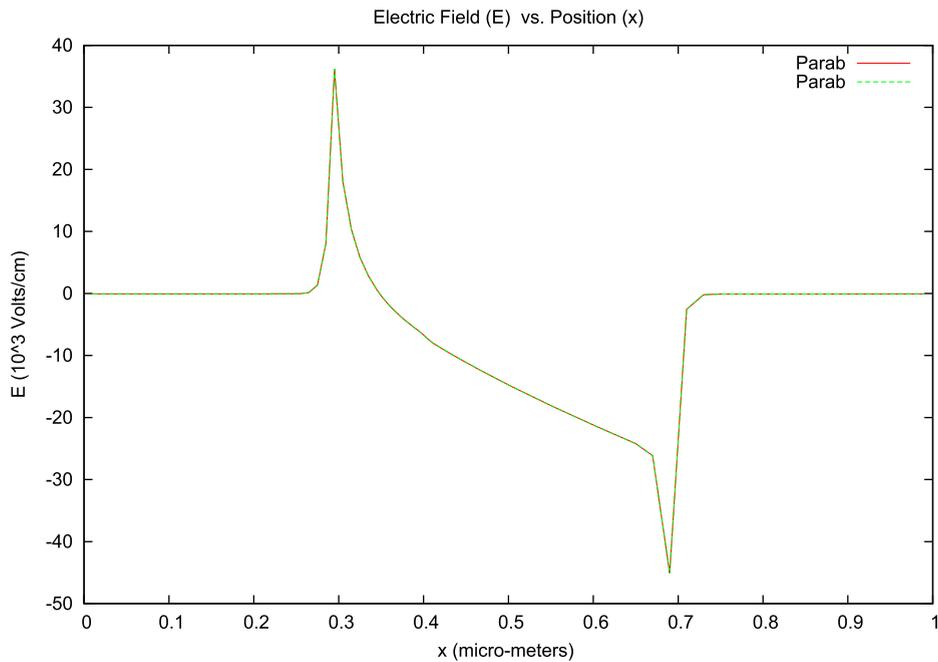
Fig. 13. Electric field  $E(x, t_0)$  for a 1  $\mu\text{m}$  diode, 0.5 V bias, and  $t_0 = 10.0$  ps.
