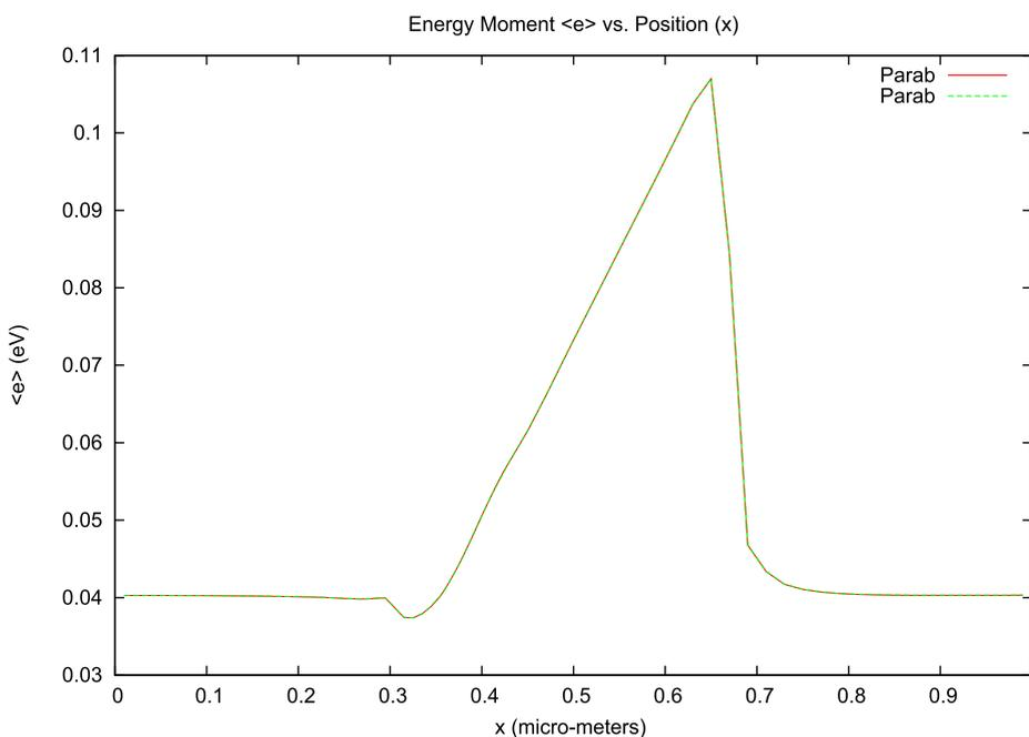
Fig. 10. Energy  $e(x, t_0)$  for a 1  $\mu\text{m}$  diode, 0.5 V bias, and  $t_0 = 10.0$  ps.
