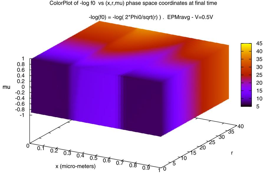
**Fig. 3.**  $-\log \alpha_0(x, r, \mu)$  for a 1  $\mu\text{m}$  diode, 0.5 V bias, and  $t_0 = 10.0$  ps.
