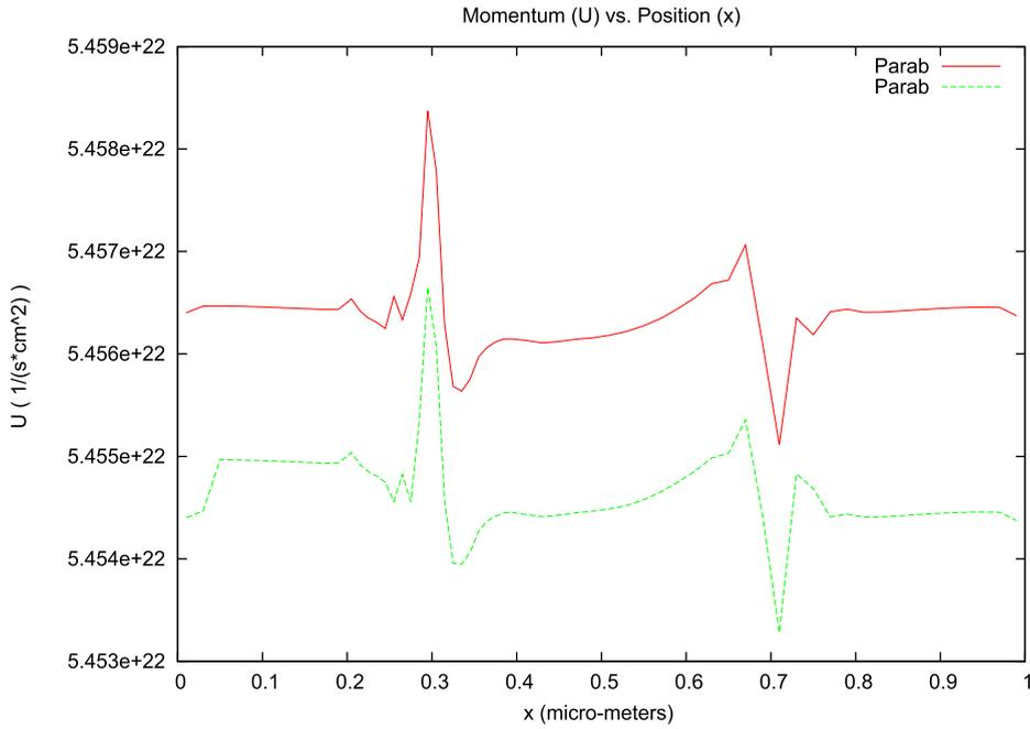
Fig. 11. Momentum (current)  $M(x, t_0)$  for a 1  $\mu\text{m}$  diode, 0.5 V bias, and  $t_0 = 10.0$  ps.
