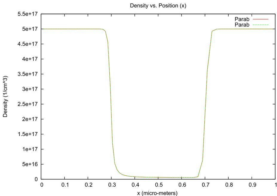
Fig. 9. Density  $\rho(x, t_0)$  for a 1  $\mu\text{m}$  diode, 0.5 V bias, and  $t_0 = 10.0$  ps.
