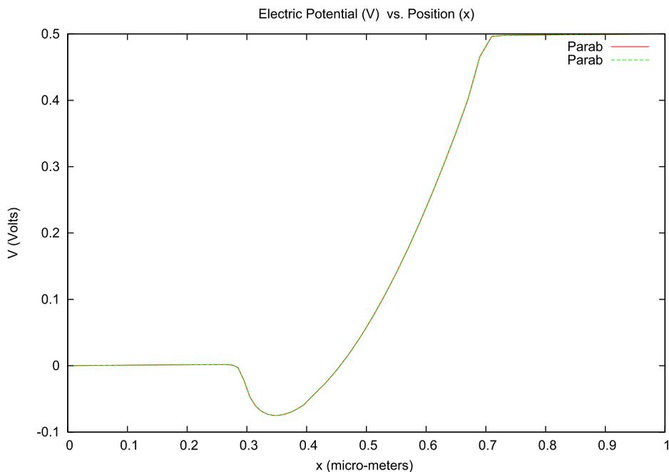
Fig. 14. Potential  $V(x, t_0)$  for a 1  $\mu\text{m}$  diode, 0.5 V bias, and  $t_0 = 10.0$  ps.
