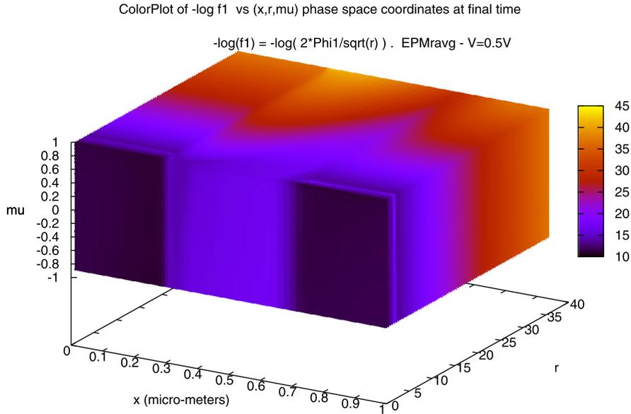
**Fig. 4.**  $-\log \alpha_1(x, r, \mu)$  for a 1  $\mu\text{m}$  diode, 0.5 V bias, and  $t_0 = 10.0$  ps.
