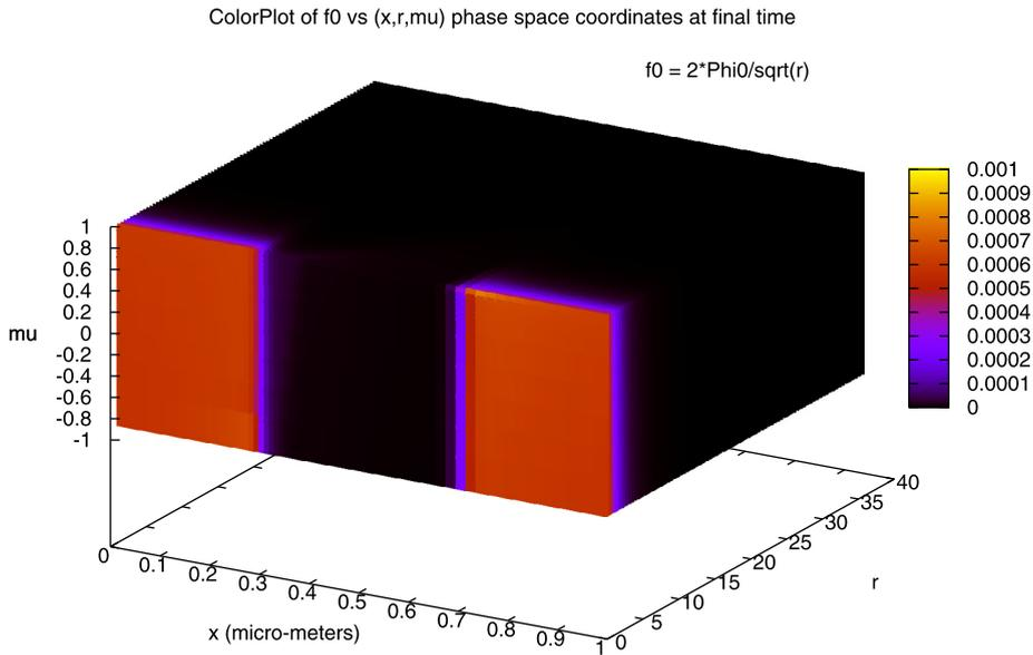
Fig. 5. Coefficient  $\alpha_0(x, r, \mu)$  for a 1  $\mu\text{m}$  diode, 0.5 V bias, and  $t_0 = 10.0$  ps.
