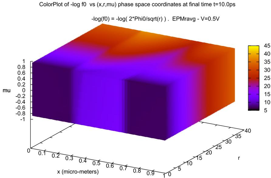
**Fig. 1.**  $-\log \alpha_0(x, r, \mu)$  for a 1  $\mu\text{m}$  diode, 0.5 V bias, and  $t_0 = 10.0$  ps. (For interpretation of the colors in the figure(s), the reader is referred to the web version of this article.)
