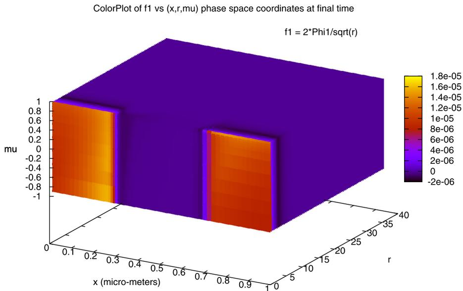
Fig. 6. Coefficient  $\alpha_1(x, r, \mu)$  for a 1  $\mu\text{m}$  diode, 0.5 V bias, and  $t_0 = 10.0$  ps.
