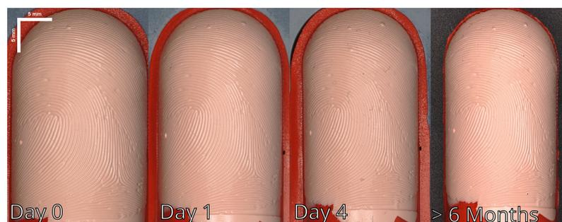
**Figure 17.** Top-down captures of created Gelafix-based fingerprint targets on different days. From left to right, day 0, day 1, day 4, and after approximately 6 months. The corresponding diameters of the fitted cylinders are summarized in Table 2. Scale bar 5 mm.
