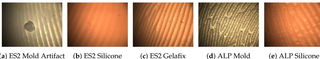
**Figure 16.** 3D-printed resin molds and fingerprint phantoms. Created with the ES2 Elegoo Saturn 2-8K resin printer (ES2) or the Alpine3D GmbH SLA service (ALP).
