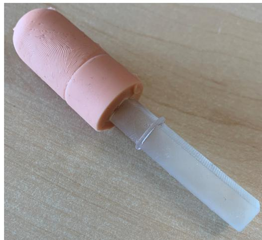
**Figure 6.** Silicone target made from 3D-printed resin mold.
