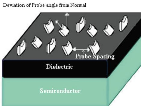
Figure 1: Schematic diagram of conventional Si BioFET structure.
